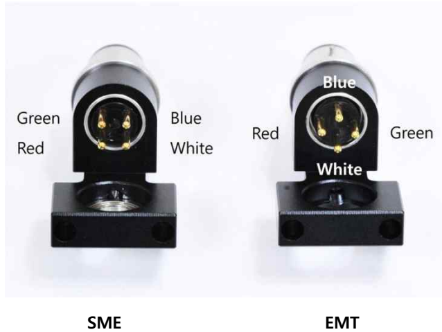
Lead wire connection
